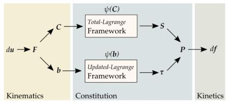
Generalized-invariants isotropic hyperelastic material formulation based on the principal stretches.
